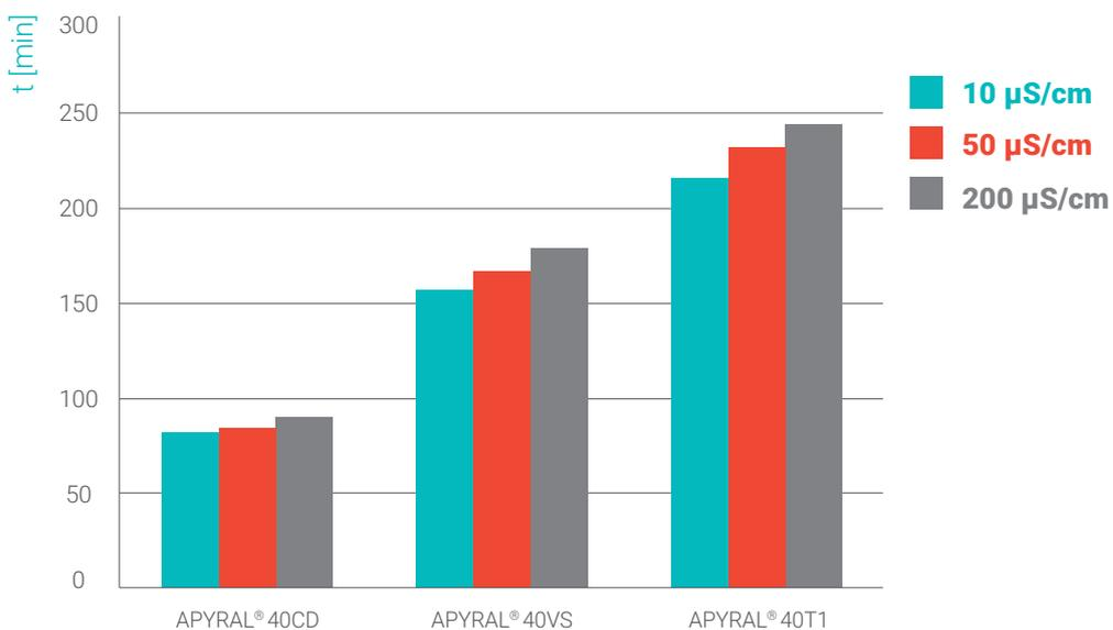
Stability measurement via dehydrochlorination (DHC) test of PVC compounds filled with 80 phr of various **APYRAL®** grades.
