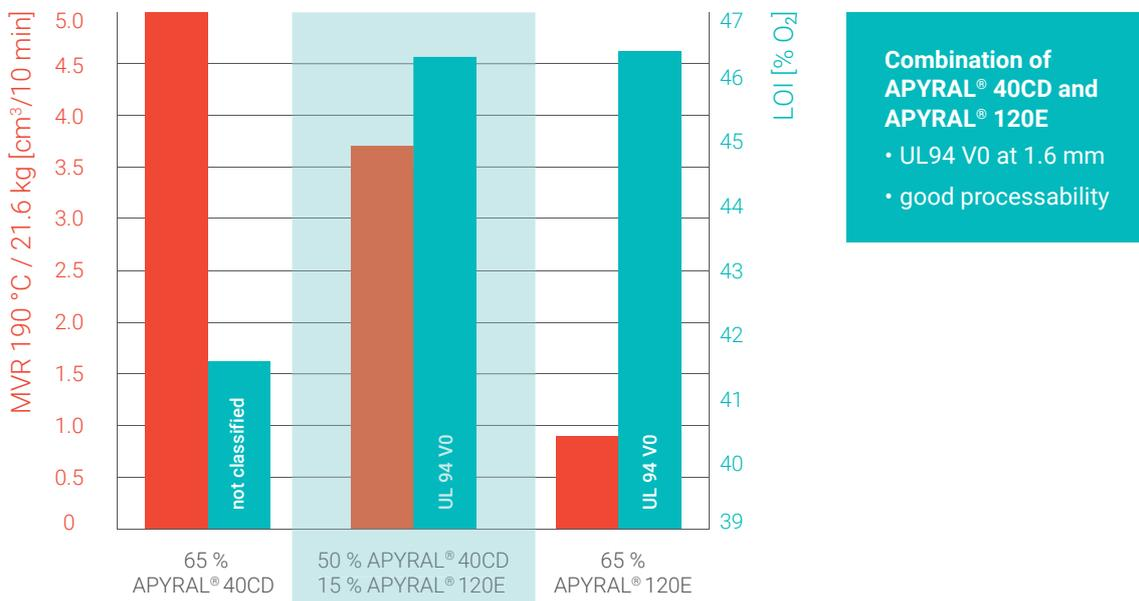
*High fire resistance* combined *with good processability*. LOI, MVR and UL94-V0 at 1.6 mm for EVA filled with 65 wt.-% **APYRAL®**.
