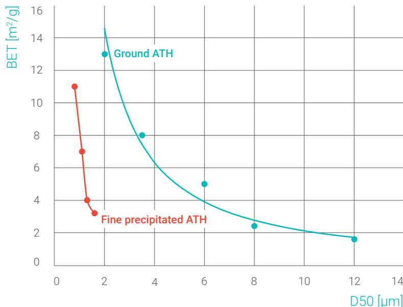
Figure 1: Correlation between D50 and BET of fine precipitated and ground ATH.
