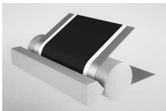
**Figure 4:** A die coating system in which the boehmite dispersion is applied to the cathode edge.
