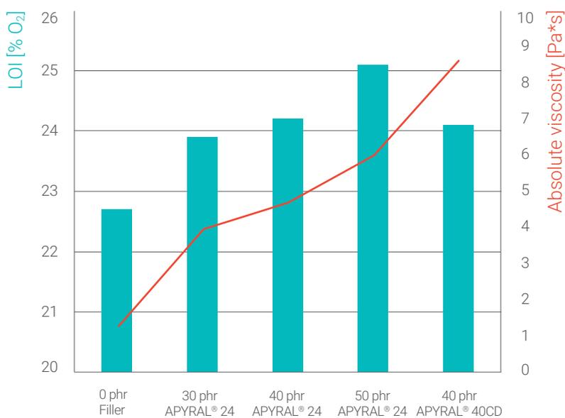
**Figure 5:** LOI and viscosity of ATH filled plastisol before curing (carried out with basic formulation given in above table with 15 phr CaCO<sub>3</sub>; without Sb<sub>2</sub>O<sub>3</sub>)
