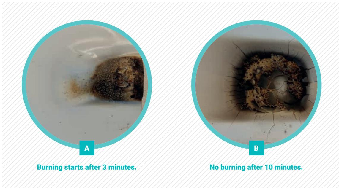
**Figure 2:** Pictures of an uncoated (A) and a coated (B) EVA sample after application of a Bunsen burner flame. Coating is an ablation coating with **APYRAL® 40CD**.
