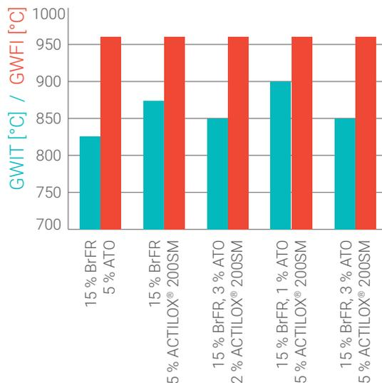
**Figure 7:** Results of GWIT and GWF1 of PA66 GF30 compounds filled with 15 % of a polymeric brominated flame retardant (Emerald Innovation 100, Lanxess) and different combinations of ATO and **ACTILOX® 200SM**.
