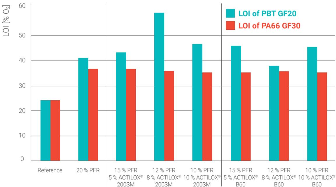
**Figure 3:** LOI values of PBT and PA66-compounds filled with different amounts of PFR in combination with boehmite (**ACTILOX® 200SM** or **ACTILOX® B60**).
