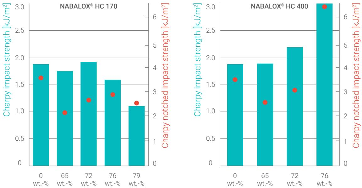
**Figure 9:** Impact strength of PA6 GF5-specimen filled with **NABALOX®** grades **HC 170** or **HC 400** after conditioning at 23 °C / 50 % relative humidity.
