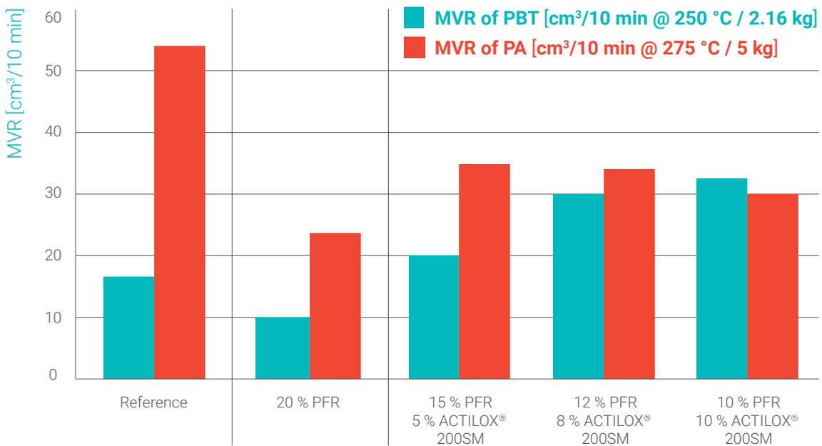
**Figure 2:** Melt volume rate (MVR) of PBT GF20- and PA66 GF30-compounds containing different amounts of PFR and boehmite **ACTILOX® 200M**. PFR = *Exolit™ OP 1200*; *Exolit™ OP 1312*.
