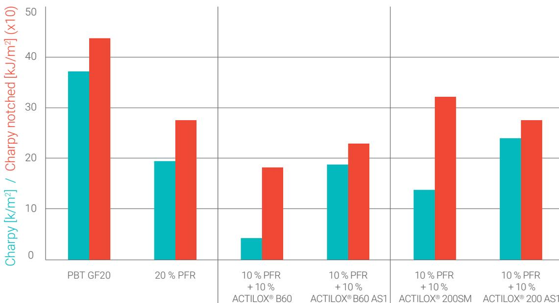
**Figure 5:** Effect on impact strength of aminosilane treated products **ACTILOX® B60 AS1** and **ACTILOX® 200 AS1** in PBT GF20 compounds.
