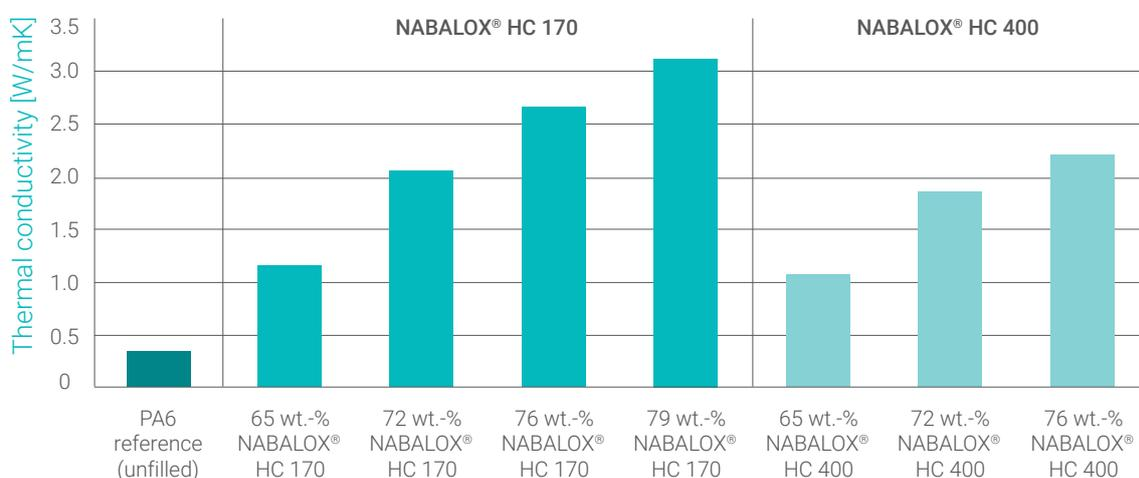
**Figure 8:** Thermal conductivity of PA6-compounds filled with **NABALOX® HC 170** or **NABALOX® HC 400**.
